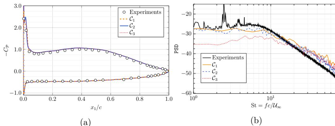
Figure 2: (left) Airfoil pressure distribution; (right) wall pressure spectrum at  $x_1/c = 0.98$ .
