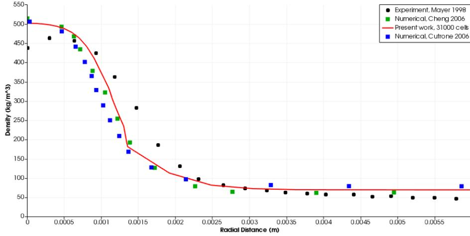
Figure 1: Density plot in supercritical cold flow case
