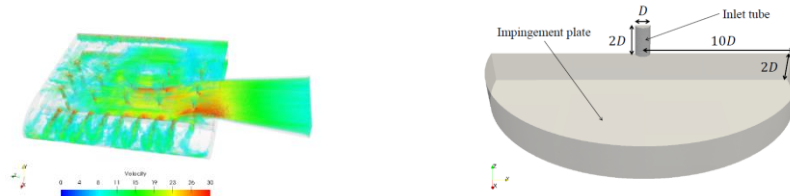
Figure 1.1 Simulation case of the 39 holes Figure 1.2 Simulation case of the single jet impingement cooling[4]
