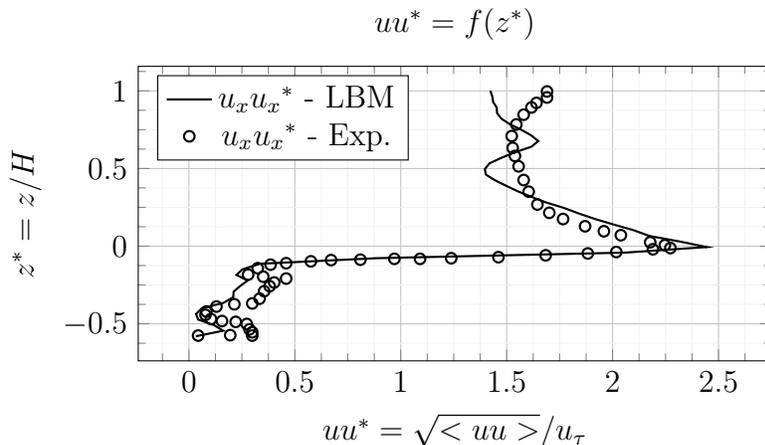
Figure 3: Average velocity fluctuations,  $x$  component.
