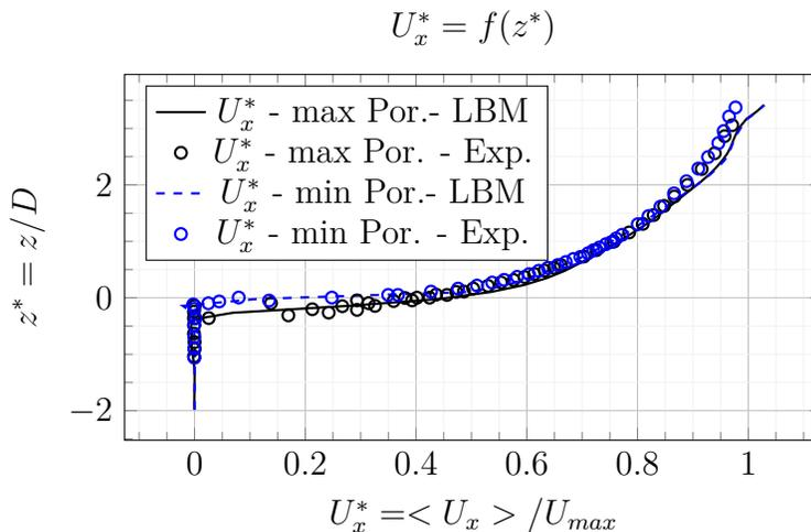
Figure 2: Average streamwise velocity in minimum and maximum porosity plane.
