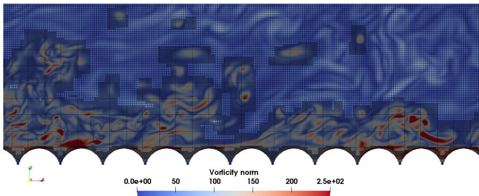
Figure 1: Instantaneous snapshot of the vorticity norm;  $xz$ -plane at  $y = H/2$ .
